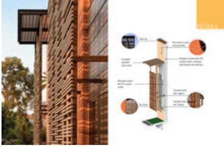
Building envelope detail showing passive systems selection - Photo Credit: Bill Timmerman
