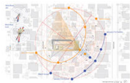
Plan organization showing relationship to sun and prevailing wind - Photo Credit: Brooks Scarpa
