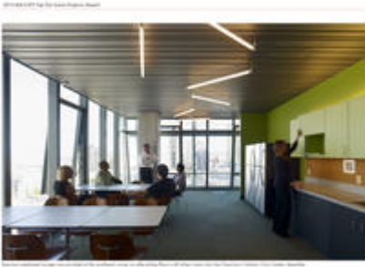
Employee lounges with views of Civic Center. All lounges have operable windows, interior light shelves and automated window shades - Photo Credit: Photographs ©2012 Bruce Damonte. All rights reserved.
